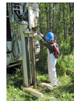
Shallow temperature survey and mapping using a Geoprobe.
